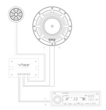
• Connect the speaker to the speaker wiring in the vehicle ensuring that correct polarity is observed.
